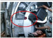
Unhopefully the ground plate's ignition marking isn't visible now. You have to either continue the marking to the motor or notice a marked point at the motor that is visible beyond the rotor.
