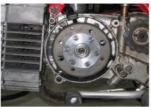
With the crank in ignition position, pull the rotor off again carefully - make sure that by doing this, you will not alter the crank position - and set the rotor again back onto the crank in such a way that the marking on the rotor aligns with the marking on the ground plate. Press the rotor on the shaft and screw it down with the original mounting screw. Make sure not to modify the crank position during this operation, otherwise you have to repeat the procedure.
