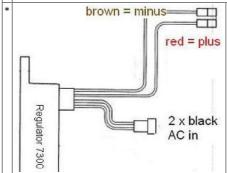
The new regulator/rectifier has 4 wires
