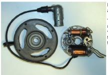
Disconnect all wires to the old dynamo, regulator and ignition coils and take those parts off.
