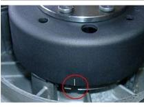
Remove the spark plugs and bring the piston to advance position. Might be 2mm BTDC.
