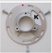
Take a look at the ground plate of the new stator (for better view it is shown without the stator). For the assembly it will be used only 3 of the 6 mounting holes (marked with screws).
