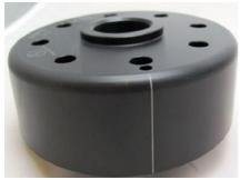
Have a look at the new rotor. You will find on its circumference a small pressed-in line. It is durable, but not well visible, so better highlighten it with some marker pen. This is also a timing mark. It will be used to align the rotor during installation.
