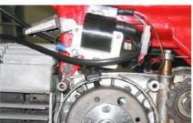
There are more than one options to mount the ignition coil. We would suggest a place close to the spark pluq.
